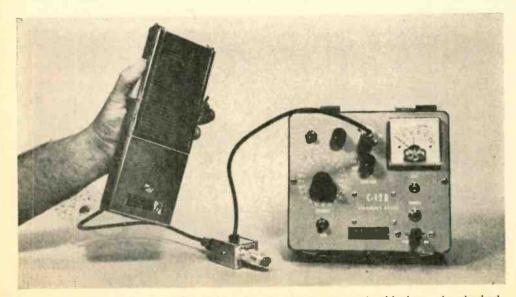
Because of their high selectivity, high-performance transceivers should always be checked with a frequency meter. Test instrument in photo above is an International Crystal C-12B.
