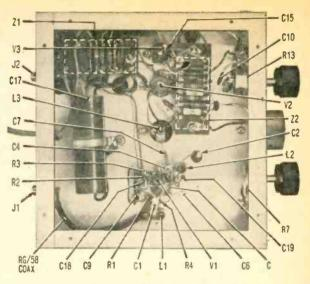
hear the characteristic superregenerative hiss from the speaker. Set the tuning capacitor (C3) to full capacity.
