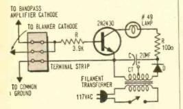
the TV receiver. The transistor is powered by a 6.3-volt filament transformer whose output is rectified by D and filtered by C. When the TV set is tuned to a color program, the bandpass amplifier and blanker cathode voltages rise because of the presence of the 3.58-MHz color burst. This provides forward bias on the transistor, causing the lamp to glow.
