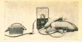
Even battery chargers have been to blame for W-T failures. Though indicator lamp on the charger above lit, charger was defective.
