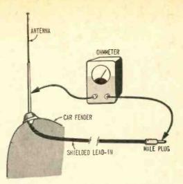
Fig. 5. Intermittent and noisy reception can be caused by antenna. An ohmmeter is the easiest way to check it for open or short circuit.
