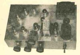
Heart of Colordaptor is this eleven-tube demodulator chassis that synchronizes video applied to pix tube cathode with disc color segments and also controls motor speed so the right color appears on screen.
