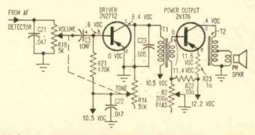
Fig. 4. Garbled or distorted sound means you should check-out the audio section; defective output transistor is very often the problem.
