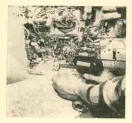
Delay line, being installed here, is used to compensate for time it takes video signal to get through Colordaptor circuits.
