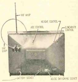
Rear view of Heath GR-104, showing position of various controls accessible through holes in cover.
