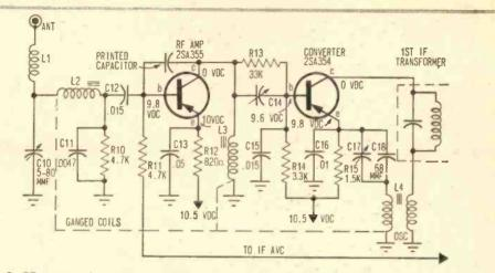
Fig. 2. RF section of typical auto radio; common defects here will often cause only local station pickup, or no stations on high end of band.
