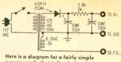
power supply that is line-Isolated. Parts values aren't critical; plate-supply voltage can be from 90 to 150 volts DC. If the transformer you use has only a 12-volt filament winding, then substitute a 12BE6 for the 6BE6 in the Dipperette-1.
