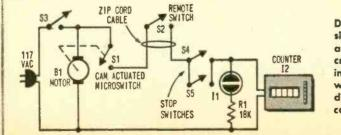
Drunkometer circuit is simple and straightforward and part location isn't critical. Timer can be used in variety of ways by substituting different control switches.
