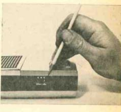
The best piece of service gear for this job is a standard 5-watt CB transceiver. Transmit a signal from the transceiver and try to receive it on the W-T. If the W-T cannot receive the signal the amplifier/modulator or receive section is at fault. Next, try using the W-T to transmit. If it works, this means the receive section is defective.
