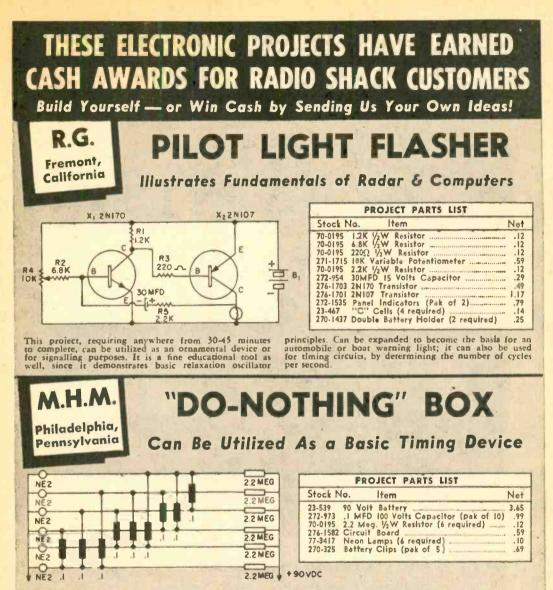
This ingenious device is a must for anyone with a keen sense of imagination. The project's most obvious feature is a series of flashing lights, which illustrate the technique of sequential lighting. The neon bulbs produce light in much the same was as outdoor display advertising. The "box" is easy to construct — at a minimum
