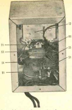
Internal layout and construction of cam-actuated microswitch can be seen above. Cam consists of small off-center knob.
