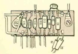
Terminal boards can be pre-assembled before mounting in chassis. Remainder of wiring is then readily completed.
