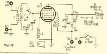
Take a good look at the schematic diagram—it's very much like the front end of a superhet. GDO coil is not part of circuit, it belongs to the grid dip oscillator that serves as the local oscillator.
