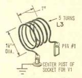
Coil L3 is wound with #16 AWG wire with an  $1\frac{1}{4}$ -in. diameter to allow most GDO coils to pass within the coil.
