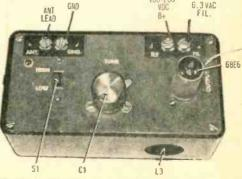
The Dipperette-1 makes a neat looking package and in a small space provided an external power source is used. The High-Low switch and Tune knob are coarse adjustments—the GDO tuning knob provides the fine tune adjust.
