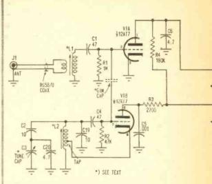
Schematic of Super Squared 3 shows low-noise triode mixer feeding superregen detector.
