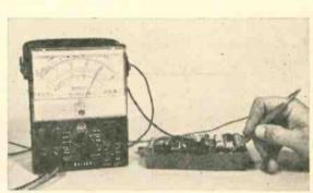
Corrosion on battery-holder terminals leads to intermittent operation, particularly if W-T is used around salt water; best cure is to sand off corrosion with fine sandpaper. Above, always check batteries under load, since output voltage can vary greatly. Batteries here registered 9V with no load, 8V on receive, 4V on transmit.
