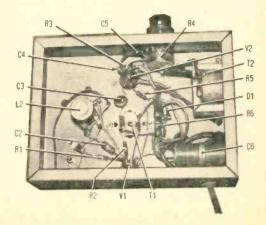
Completed wiring of BCB 2 shows few parts and wide-open spaces making construction a snap.
